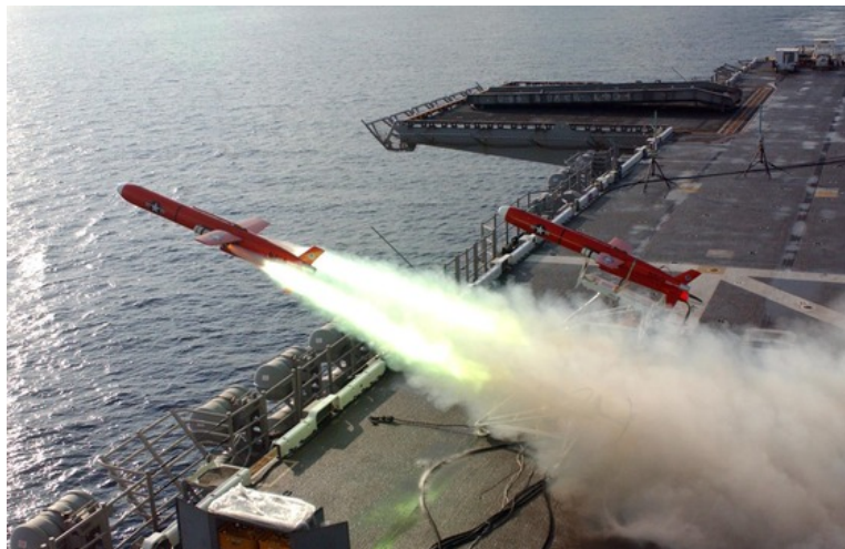
A BQM-74E aerial target drone launches from the flight deck aboard the amphibious assault ship USS Boxer (2005). US Navy photograph by Photographer's Mate Airman Paul Polach / Wikimedia Commons
